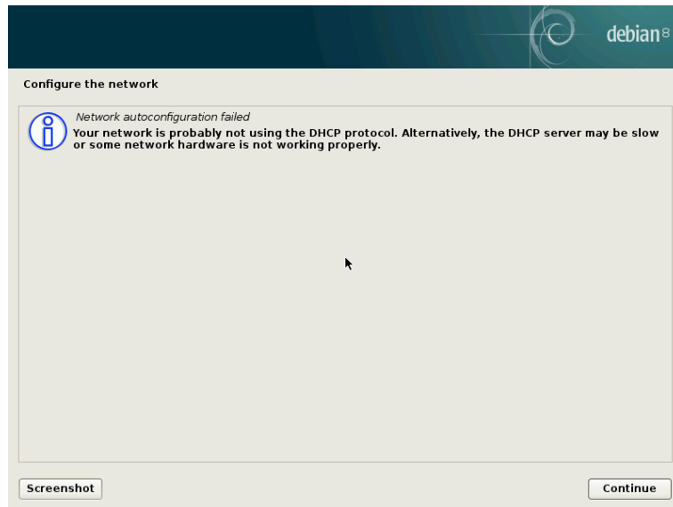
Fig. 6: DHCP configuration failed
